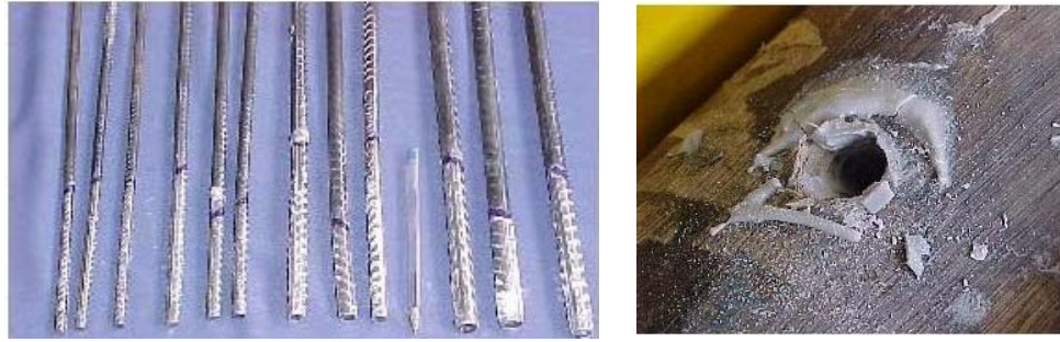
Figure 7. Shapes of rupture, regardless diameters and lengths of anchors
