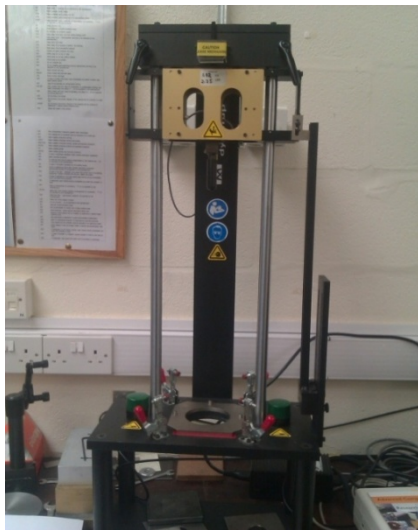
Figure 4. Impact Machine, drop weight ( Adopted from: UoB. 2012)
