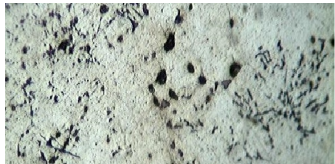
Figure 4. Optical micrograph of T6 Tempered Al-Zn-Mg-Cu alloy, x200
