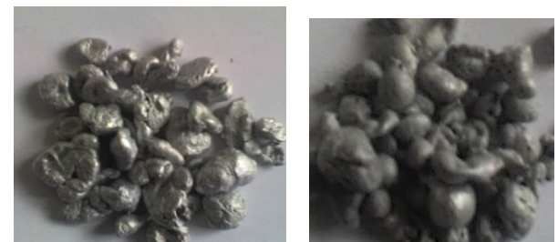
Figure 8. Amorphous aluminium balls produced at 52cms -1 cooled in (a) water (b) brine
