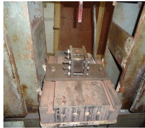
Figure 2. Die assembly mounted on 25 ton Hydraulic pressing machine
