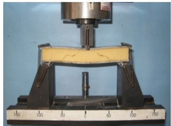
Figure 2. Specimen during fatigue testing
