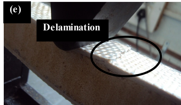
Figure 11. Failure of high density sandwich composites
