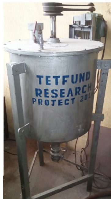
Figure 1. Diagram of the Constructed Digester
