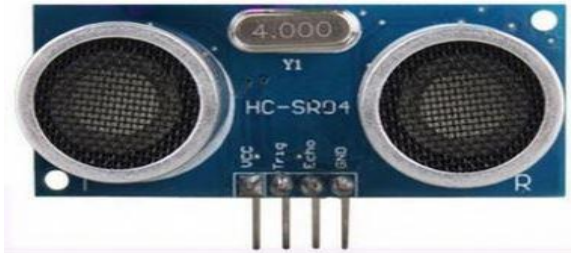
Figure 2. The HC-SR04 ultrasonic proximity sensor
