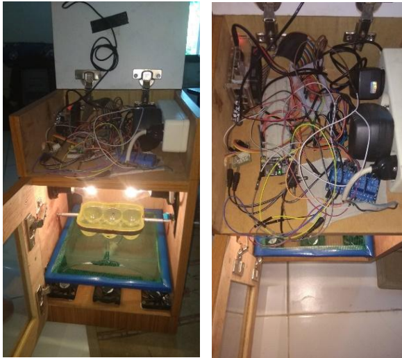
Figure 4. Prototype of chicken eggs incubator machine from inside
