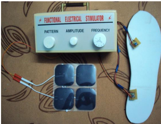
Figure 5.2. Complete set up of the portable functional simulator
