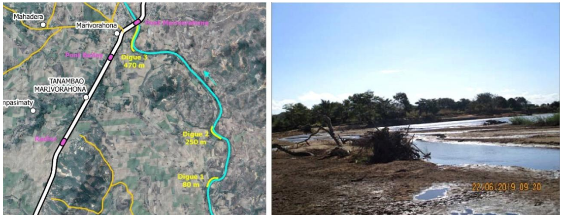
Figure 2. Left: location of the left bank embankment dikes. Right: photo of the breach at the location of Dike 1 [3]
