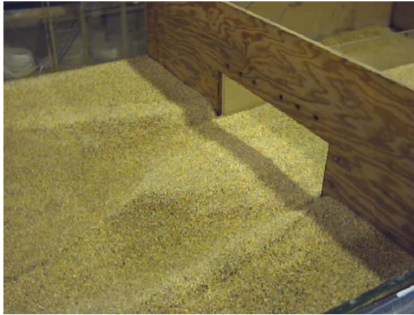
Figure 1. Culvert outlet, no wingwalls
