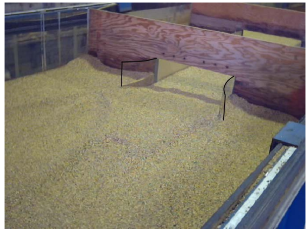
Figure 6. Culvert outlet, short streamlined beveled shaped (plexiglass) wingwalls
