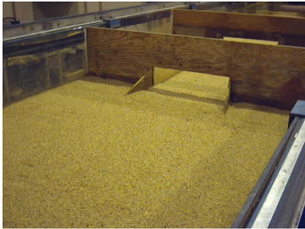
Figure 2. Culvert outlet, 8 degree rough (wood) finish wingwalls
