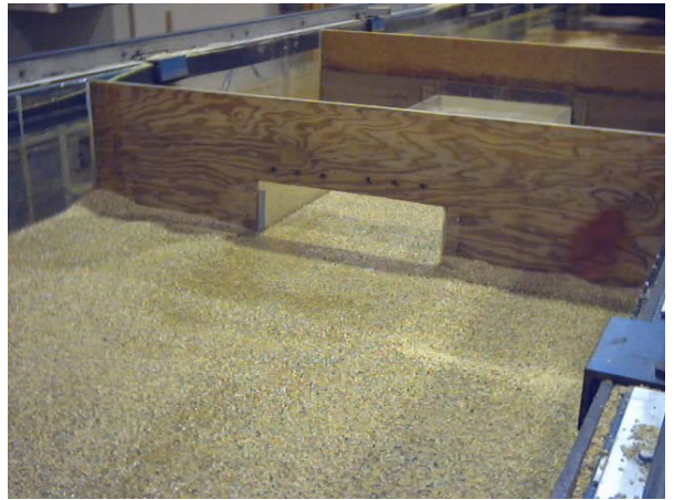
Figure 5. Culvert outlet, truncated circular beveled shaped (plexiglass) wingwalls
