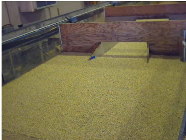
Figure 3. Culvert outlet, 8 degree smooth (plexiglass) finish wingwalls
