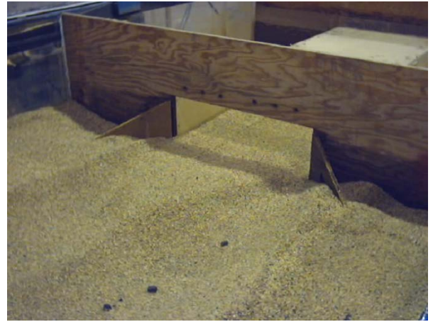
Figure 4. Culvert outlet, 45 degree rough (wood) finish wingwalls
