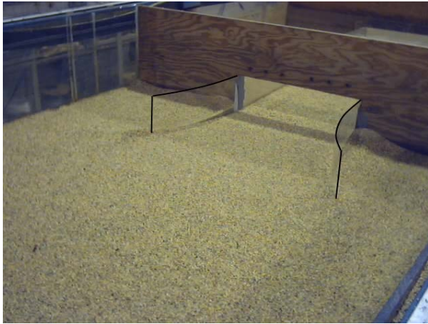
Figure 7. Culvert outlet, long streamlined beveled shaped (plexiglass) wingwalls
