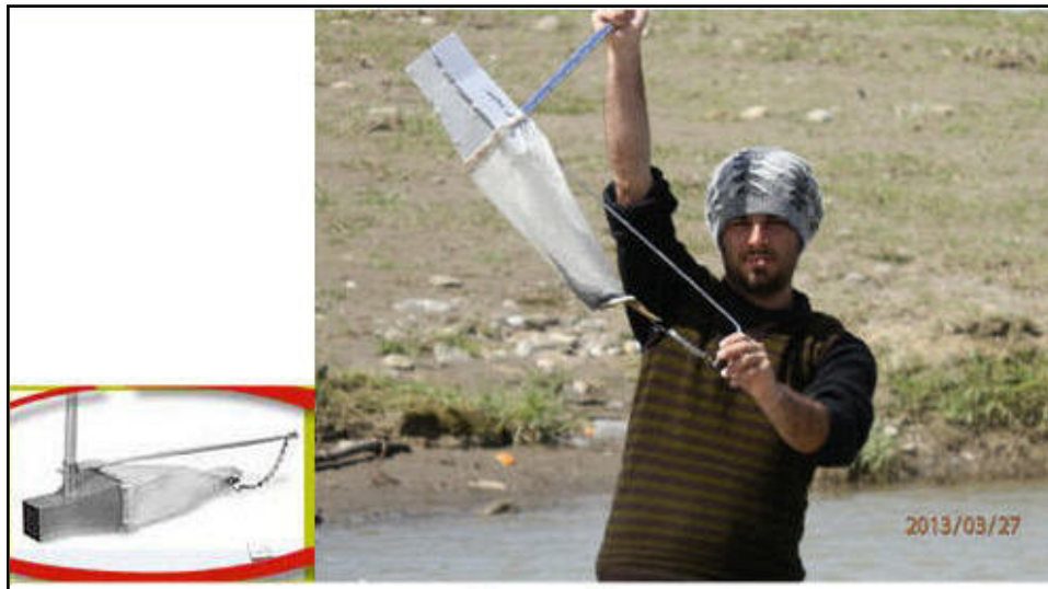
Figure 5. Helley-Smith sampler
