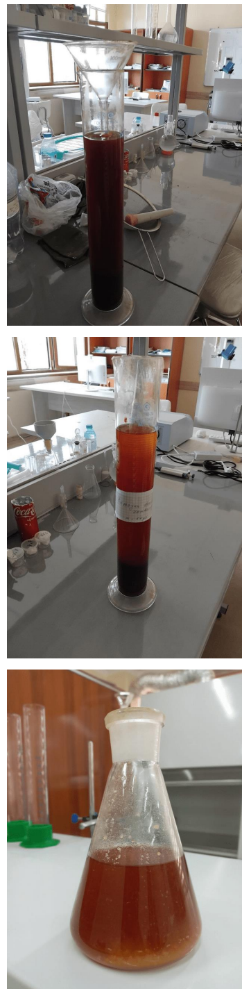
Figure 2. Filtration of the 96% ethanolic extract prepared from 54 g of dried I. hispidus biomass
