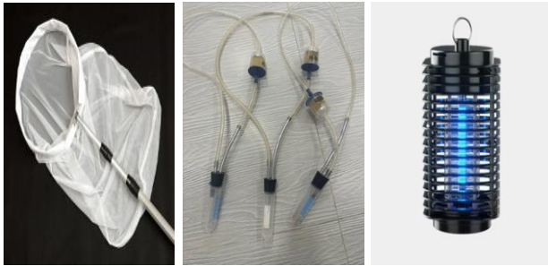
Figure 3. Equipment used for collecting insects (A. Entomological net, B. Exhauster, C. Light trap)
