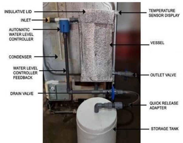
Figure 2. Rear of the Refrigerator installed with Heat Extraction System
