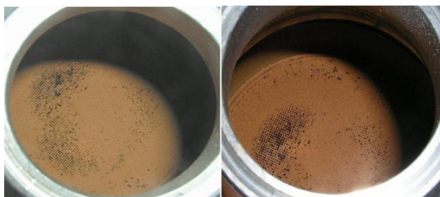
Figure 4. Catalyst frontal area: 90% blocked (manganese content of deposit: 75%) [8]
