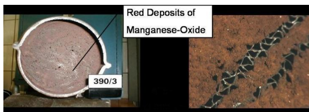
Figure 1. Deposits of manganese oxides on a catalytic converter operated in a vehicle from the Chinese market (front surface and detail) [8]
