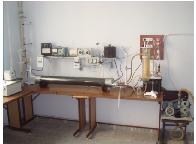
Figure 1. General view of solar heat-exchanging – solar reactor accumulating system in laboratory condition
