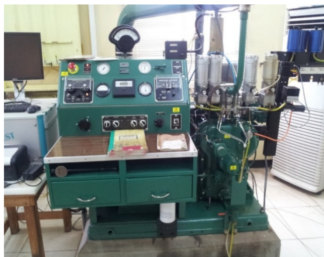
Figure 1. Cooperative Fuel Research (CFR) Engine
