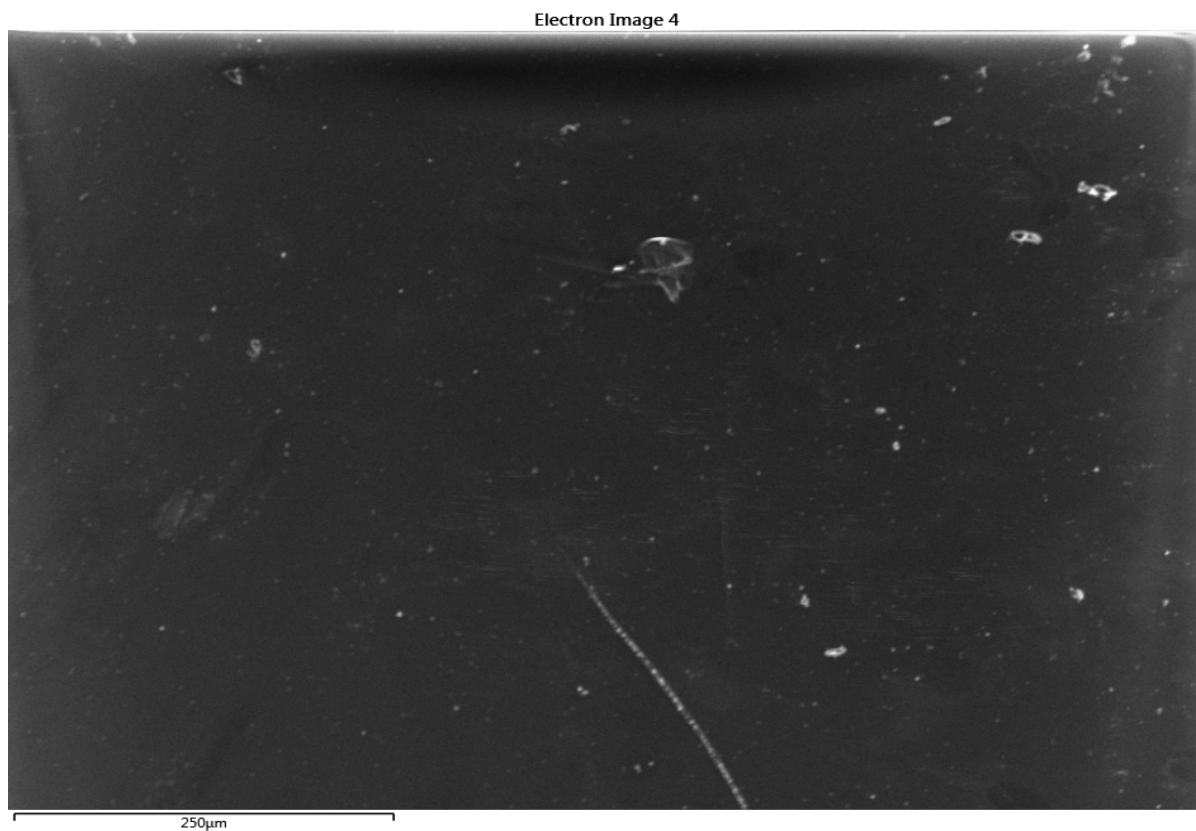
Figure 3. 120μm SEM micrograph of uncleaned glass substrate @120 magnification (scale bar: 250μm)
