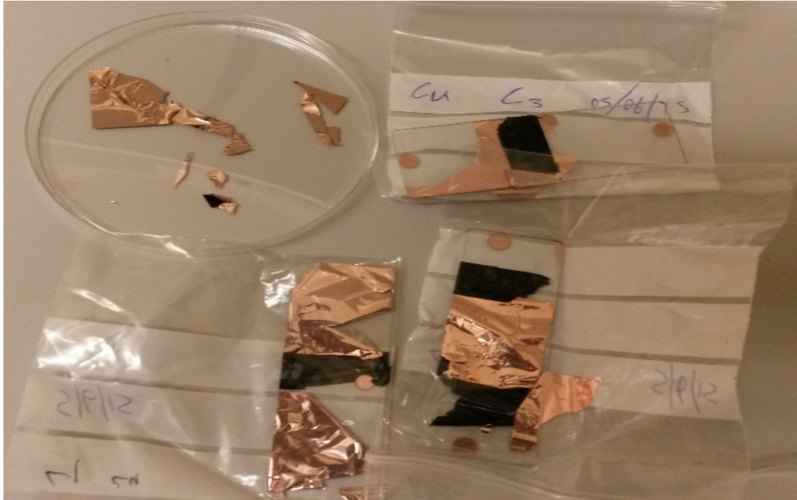
Figure 10. Copper coating delamination at 1700 nm film thickness
