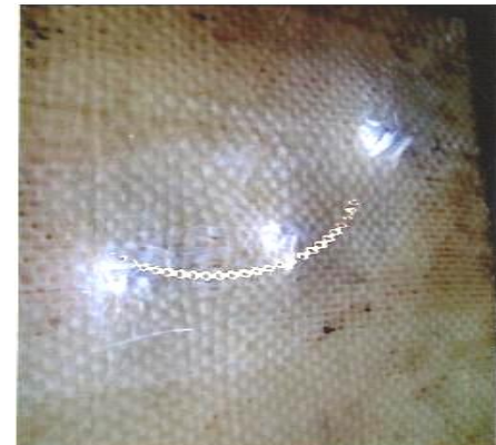
Figure 3. Sample D, showing minimal shattering by impact
