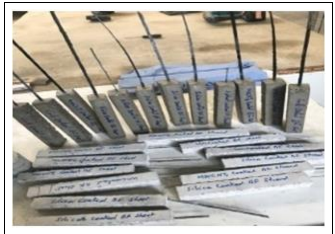
Figure 2. Coated and uncoated basalt fiber strand and sheet specimens
