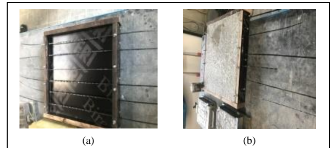
Figure 1. Photograph shows that (a). coated and uncoated basalt fiber strands/sheets under tension in the mold, and (b). concrete, sand and cement mixture poured in molding box.
