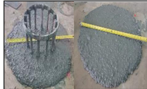
Figure 2. J-ring and flow test of LW-SCC
