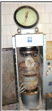
Figure 5. Splitting tensile Strength test
