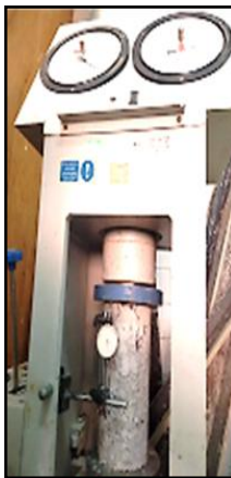
Figure 4. Modulus of Elasticity test
