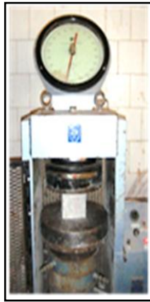
Figure 3. Compressive Strength test
