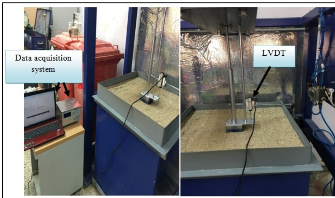
Figure 7. Linear variable differential transformer (LVDT)
