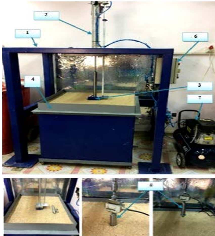
Figure 1. General view of the manufactured apparatus: 1-Loading steel frame, 2- Axial loading system, 3- Model footing, 4- Steel container, 5- Cone and shank, 6- Control system, and 7- Air compressor system
