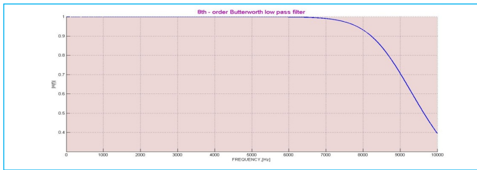
Figure 12. Frequency response of 8th order Butterworth low pass filter
