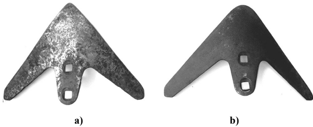
Figure 7. Cultivator plowshares after 25 ha of operation, consolidated by: a - reload laser of alloy PS-14-60 + 6% B 4 C (proposed technology), b - induction welding of alloy PS-14-60 (basic technology)
