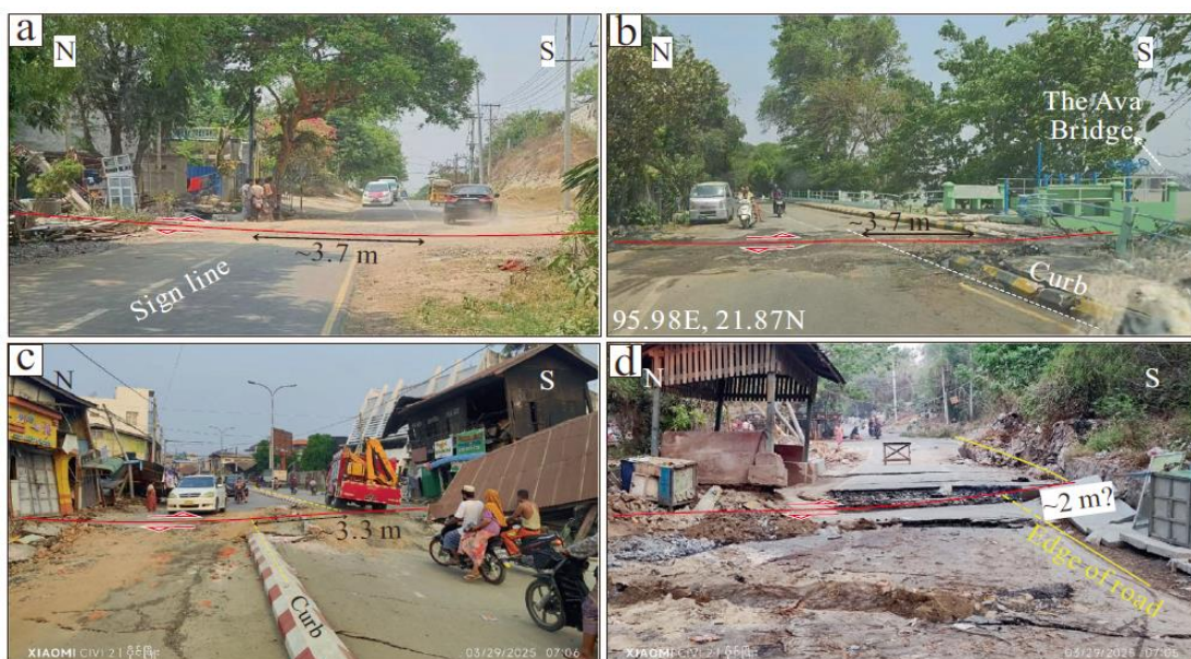
Figure 6. Field photographs of the coseismic slips of the earthquake surface rupture zone along the SSF (Source: Twitter account @heungburma). a–d represent coseismic slips measured from offset roads at four different sites
