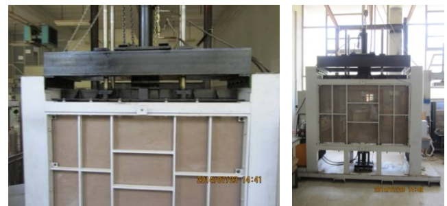
Figure 8. Loading Jack to apply surcharge
