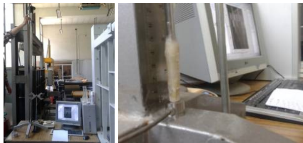
Figure 6. Calibrating the stress sensors
