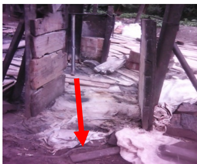
Plate 3. Floor of manual cassava paste press having direct contact with soil
