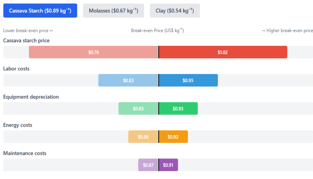
Figure 2. Tornado diagram of break-even price sensitivity ( \pm 20\% variation). Whiskers denote 5th–95th percentile from 10 000 Monte-Carlo runs
