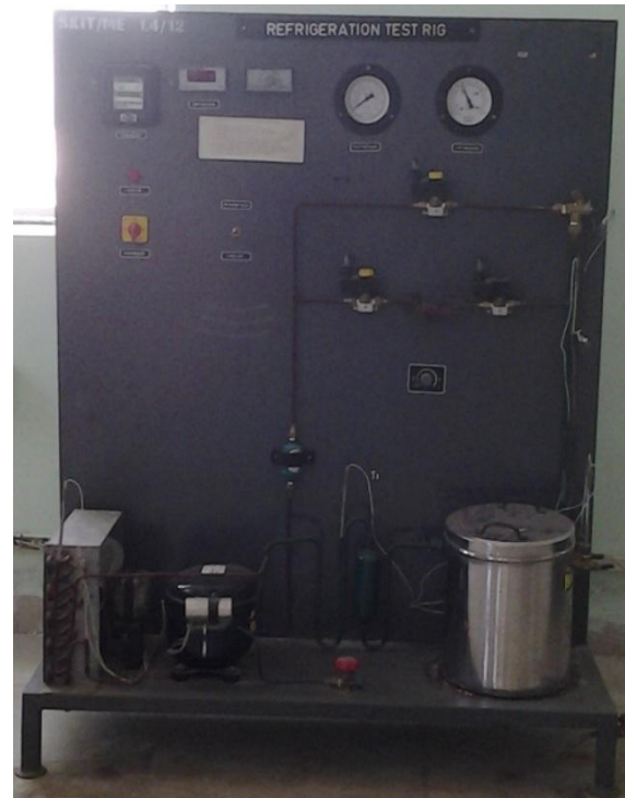
Figure 1. Experimental set up (Refrigeration Test Rig)
