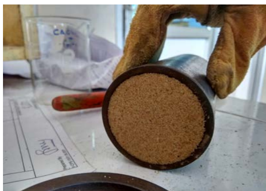
Figure 1. Cylindrical Specimen in Compression Pattern
