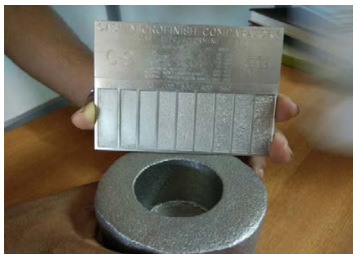
Figure 8. Casting analysed with the help of comparator
