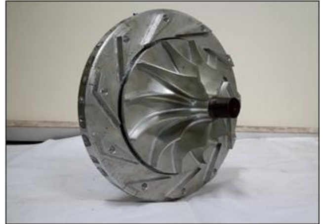
Figure 8. Assembly of Impeller and diffuser
