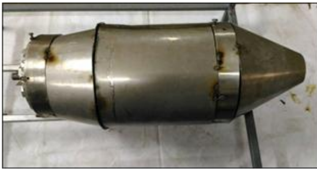
Figure 11. Turbojet engine complete assembly
