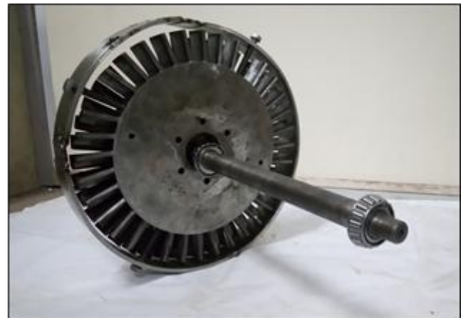
Figure 9. Assembly of Stator, Rotor and the shaft
