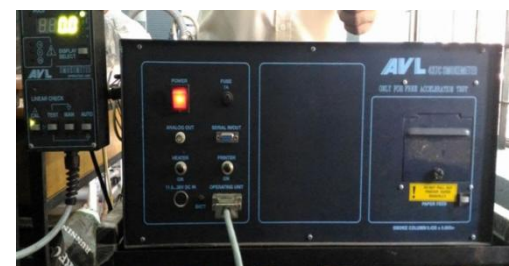
Figure 5. Smoke indicator
