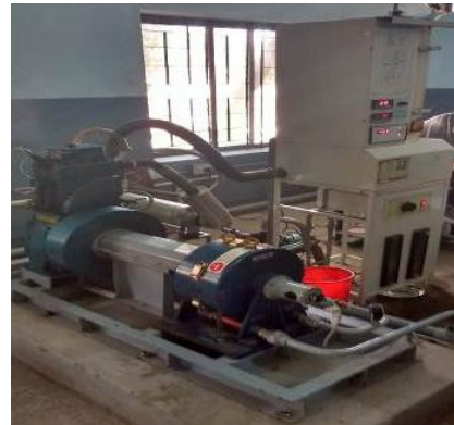
Figure 3. Diesel engine test rig
