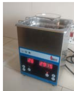
Figure 2. Blending of biodiesel with silver nanoparticles in ultrasonicator
