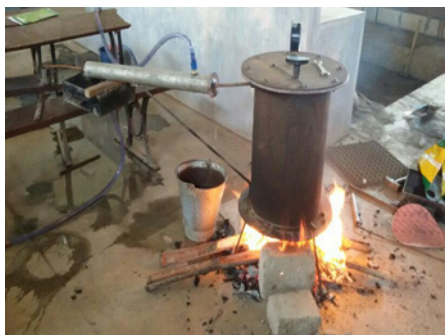
Figure 1. Working of Pyrolysis unit
