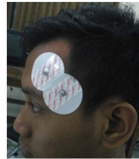
Figure 12. Electrode position on the forehead for the forward movement
