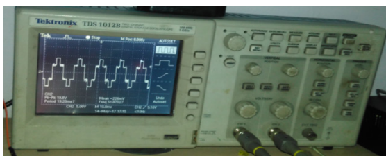
Figure 13. Three phase line-line inverter voltage
