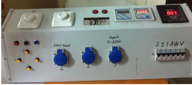
Figure 4. Isolated and regulated power supply circuit
