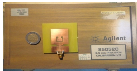
Figure 6. The achieved broadband antenna
