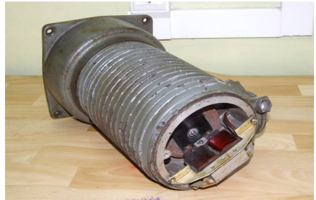
Figure 3. View of motor with integrated construction from non-demountable bearing shield
