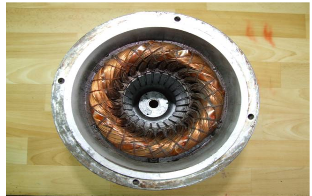
Figure 4. Interior view of the stator of the electric motor
