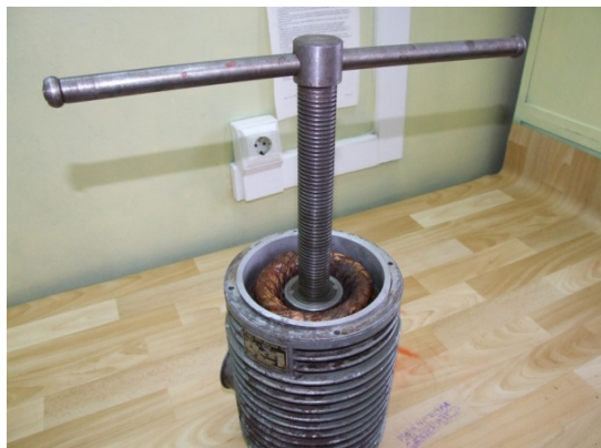
Figure 9. The extraction device in working position
