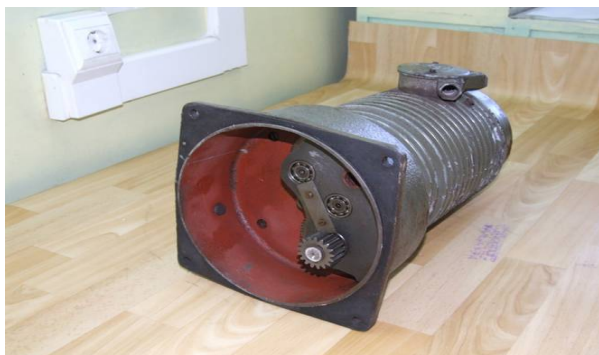
Figure 2. View of motor with integrated construction from demountable bearing shield
