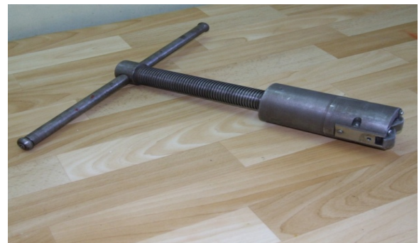
Figure 7. The extraction device, before the insertion into the stator
