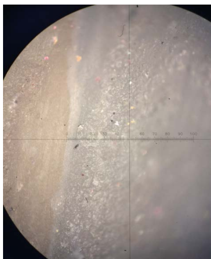
Figure 2. Fifty micrometer marginal fit under stereo microscope X 10
