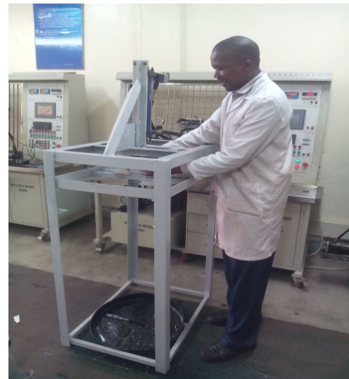
Figure 4. Positioning of the forming box on the hydraulic press ready for operation
