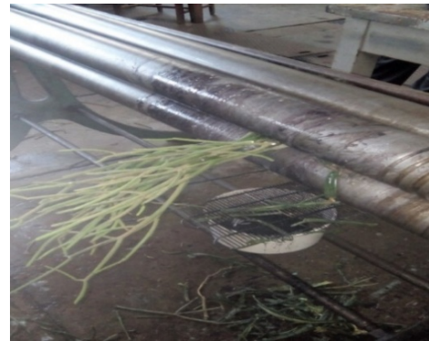
Figure 3. Extraction of euphorbia sap using a sheet rolling machine
