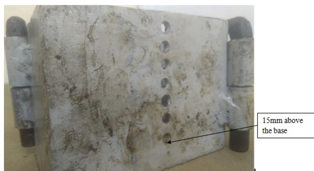
Figure 5. Forming box with inspection holes on the side
