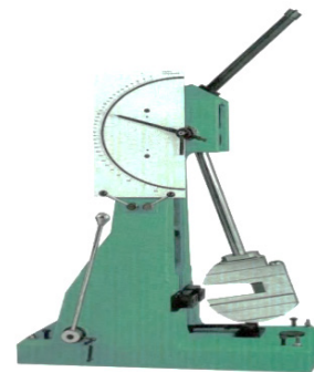
Figure 5. Charpy Equipment
