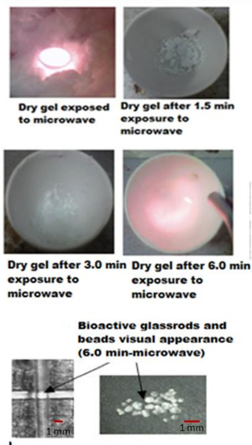
Figure 1. Visual appearance of the bioactive glass 45S5 synthesized by sol gel method using microwave for dry gel stabilization. 1.5 and 3 minutes exposure were not enough to melt the sample and obtain translucent glass
