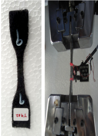
Figure 4. Specimen (a) before testing (b) during testing
