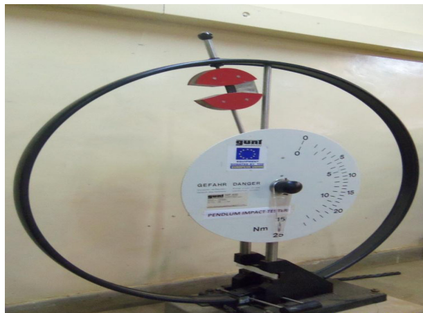
Figure 3. Specimen under Impact test
