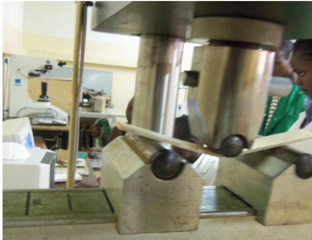
Figure 2. Specimen under bending test
