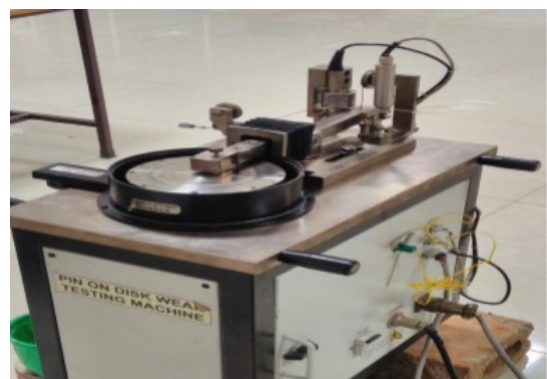
Figure 5. Pin on Disc Apparatus
