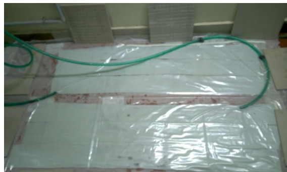
Figure 1. Vacuum Bagging Method
