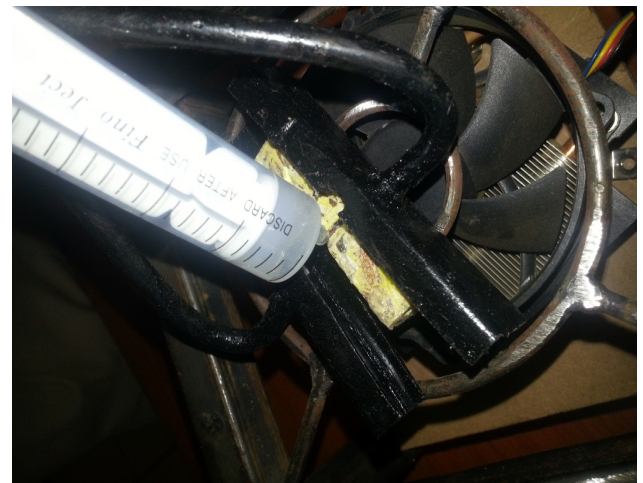
Figure 3. Healing set up when using draught fan
